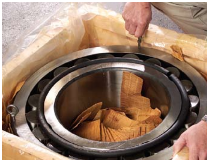
Fig. 2 Eyebolts can be inserted into lifting holes
