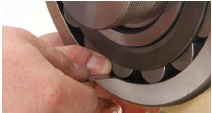
Fig. 31 During mounting, the RIC should be checked at the unloaded roller
