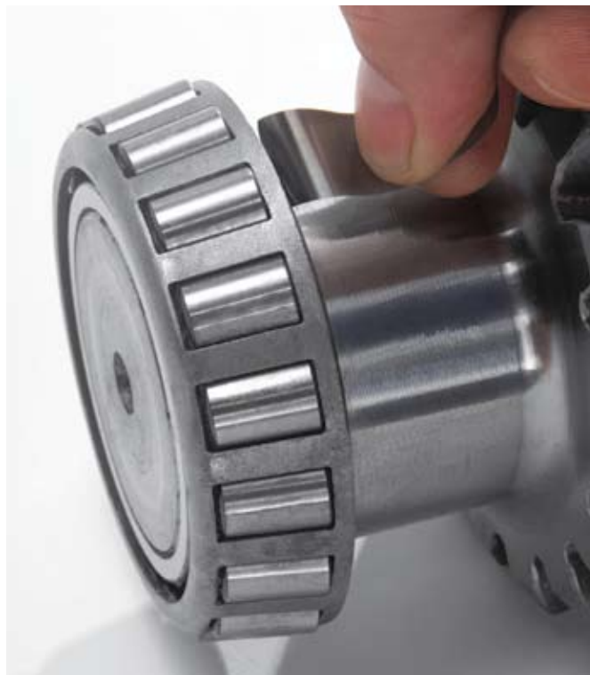
Fig. 23 Bearings should be checked with a feeler gage to ensure proper fit
