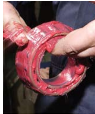
Fig. 61 Grease can easily be packed by hand
