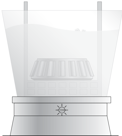
Fig. 6 Bearings can be heated in a pan or metal container filled with oil
